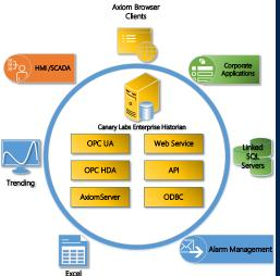
The Enterprise Historian Data Mirror provides customers with the ability to transport real-time and snap shot images of data from a primary historian to a secondary historian. The secondary historian can be on the same network but installed on a separate PC for disaster recovery purposes or the data could be transported via the web to a facility at another physical location.
